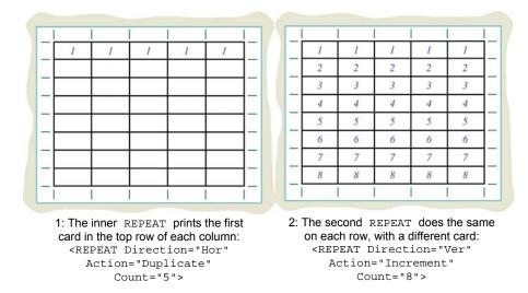
**Printing pre-sorted stacks:** If the attribute values are *Direction="Stack" Action="Increment"*, **REPEAT** puts the next Signature on the next sheet. That is, the signatures will repeat through the stack of sheets, producing a stack of pre-sorted documents.
