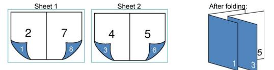
The cell assignments shown in the above diagram for the eight pages are as follows. Pages that get assigned to the second signature are shown center-aligned so they're easy to recognize; notice that within each signature, the page sequence (as shown in the illustrations) is Down Up Up Down.
