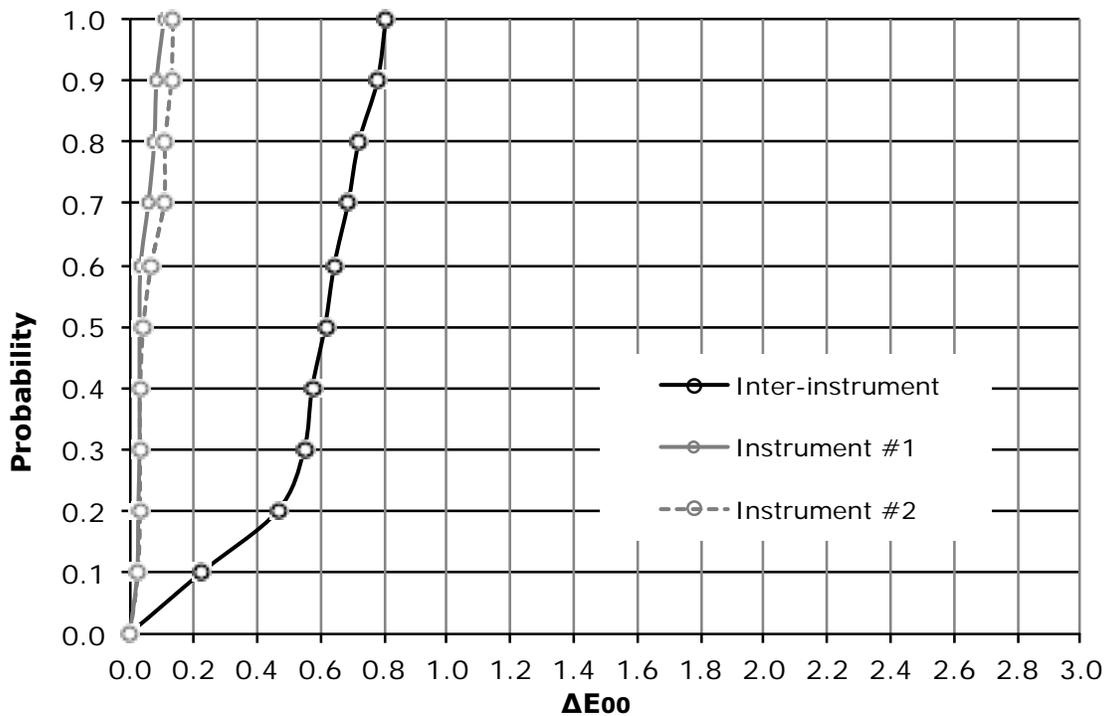
Figure B.1 Repeatability and the inter-instrument agreement between Instrument #1 and Instrument #2
